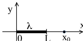
a) (9 pts) Calculate the electric potential  $V(x_0,0,0)$  at some given arbitrary point “ $x_0$ ” on the positive  $x$ -axis (assume  $x_0 > L$ , i.e. we are past the end of the charged rod)
